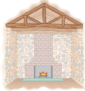
FIGURE 12–26 A roof truss.
